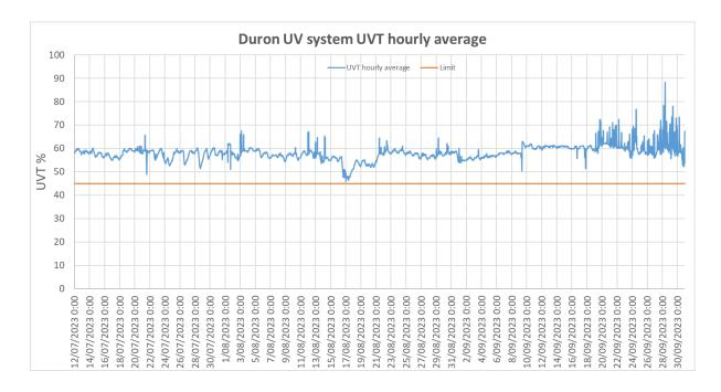
It has been noticed that the UVT readings are not reliable and have fluctuated significantly since the 19th of September as shown above. The instrument supplier was on-site investigating, and they have recommended some improvements such as moving the UVT probe from the UV channel to the pre-UV channel, and installing the instrument in a horizontal position which might provide a more representative reading.
